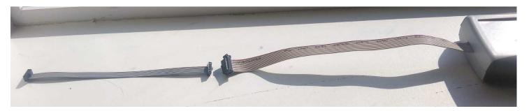
Near the center of the image, using scissors, cut off the two black connectors. With the same scissors, cut carefully between each wire, separating them into individual wires. Wearing nitrile gloves, strip and twist each wire in preparation for mating/soldering. A diagram below will show the exact mating, but when you are done it will look like this:
